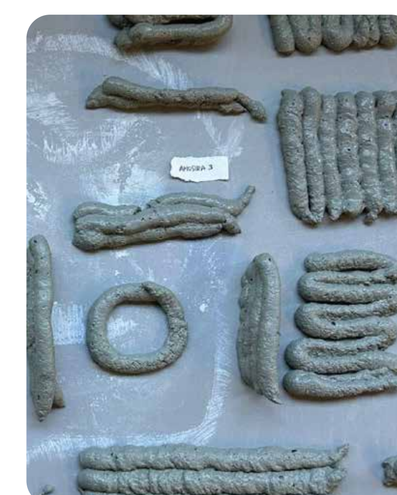
Figure 2. Testing mortar proportions for the extrusion process. Gabriel Monteiro and Ilse Matus images, 2024.
